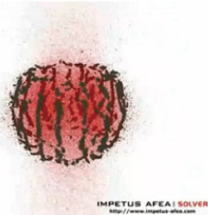
Fragmentation of metal cylinder following high explosive (C-4) detonation
